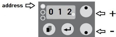
If all 3 numbers are fixed, the address is confirmed. The picture above shows address No. 12.
