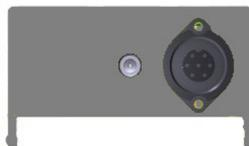
At the back there is the main power switch and the charging socket.
