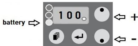
In standby (sleep) mode the display is OFF, right decimal point is still ON to show that ptx RM is ready to operate.
